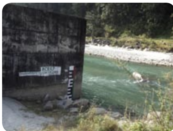
Figure 3.9: River Water Level Gauge in Dolakha, Nepal
